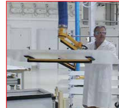
Mechanical gripper as undergripper for glass panes
