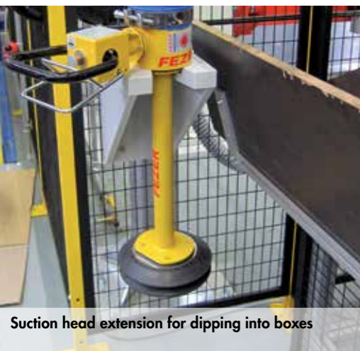
Suction head extension for dipping into boxes
