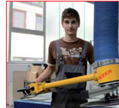
Extension for control housing for large-sized workpieces
