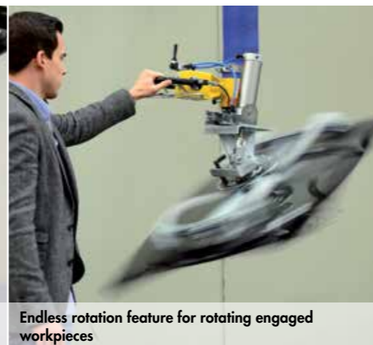
Endless rotation feature for rotating engaged workpieces
