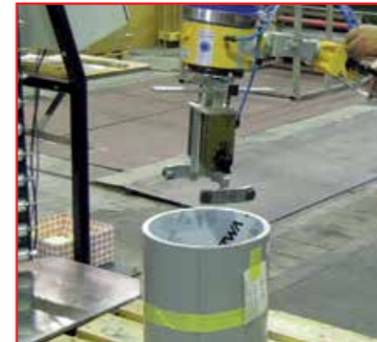
Pneumactical gripper for handling coils or tubes
