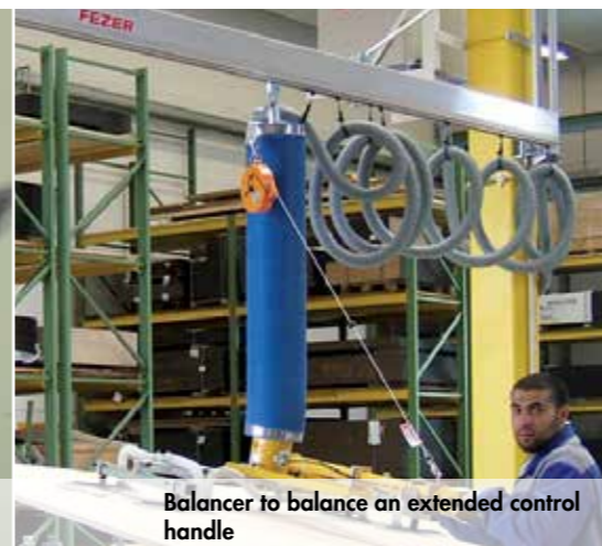
Balancer to balance an extended control handle
