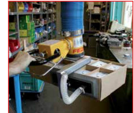
Special suction foot for lateral engagement of cardboard boxes
