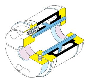
The 715/PG air chuck is recommended for unwinding and rewinding with cores. The body of the chuck can be either light alloy or steel, whereas the expanding section is made of a high-resistance rubber band. It is available with side flange for mobile arms unwind stand mounting, or with a passing bore for passing bars mounting. The steel clamp grants a perfect gripping onto the bar and can be replaced with fixing grains to reduce down the weight.
