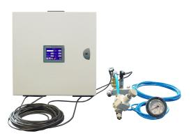
The System is made up of a control unit designed for managing Leak Testing process of Containers, Human Machine Interfacing, and pneumatic actuators. It can be equipped with one or more Testing Chamber under Vacuum or Pressure. Leak Testing process starts when the Cycle Start button is pressed. Test result (Conforming or Non-Conforming) is displayed on the HMI screen.
