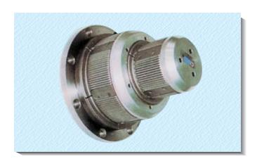
The Model 711/MA is recommended primarily for unwinding of both steel and cardboard cores. It is superior for higher weight, speed and grants a perfect core centering. The body of the chuck and the expandors (leafs) are available in steel only. The flange mounting is always custom-made and the chuck can be stepped for use with different core sizes. The expanding elements, pin-fitted on a cam, are expanded through the reel rotation combined with the web tension.
